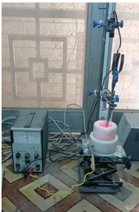
Figure (2.1): Photographic image photo-electrochemical etching set-up.
