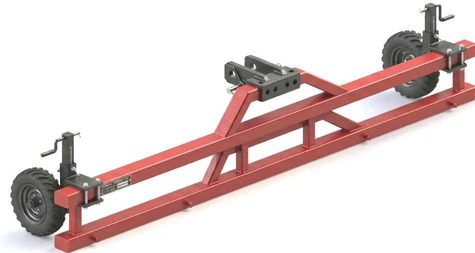
Figure 1. Three-dimensional (3D) computer model of the support frame of the improved tiller.
