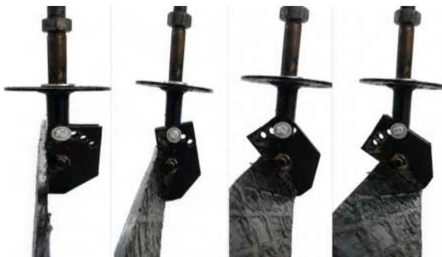
Figure 3. Installation angle of soil pushers relative to the vertical at angles of 30, 35, 40, and 45°
