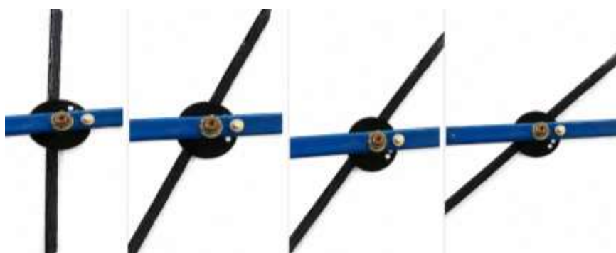
Figure 2. Installation of soil pushers at angles of 25 (a), 30 (b), 35 (c), and 40° (d) relative to the direction of movement
