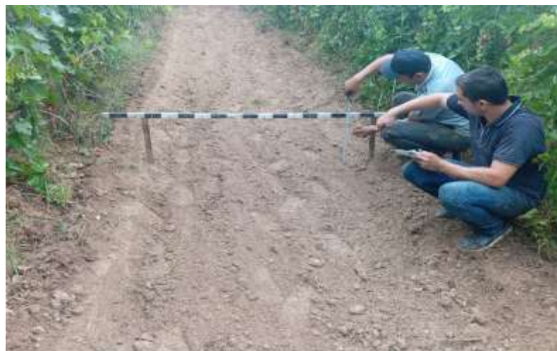
Figure 5. Obtaining the transverse profile of the cultivated field surface on a device equipped with levelers
