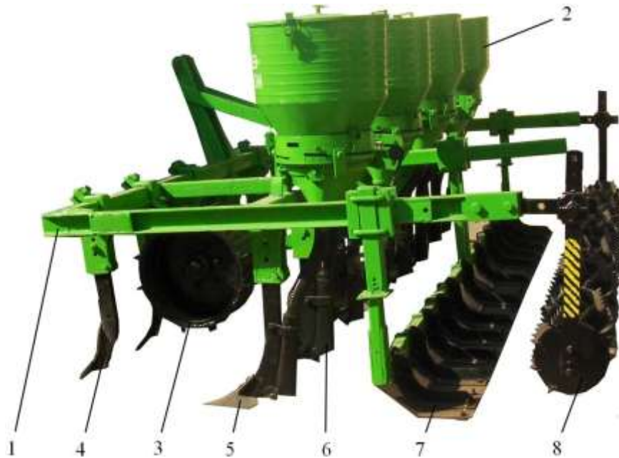
Figure 3. KM-3.0 combined machine: 1 – frame; 2 – fertilizer spreader; 3 – base wheel; 4, 5 – soil softening working bodies; 6 – coulter; 7 – leveler; 8 – toothed-plank reel.
