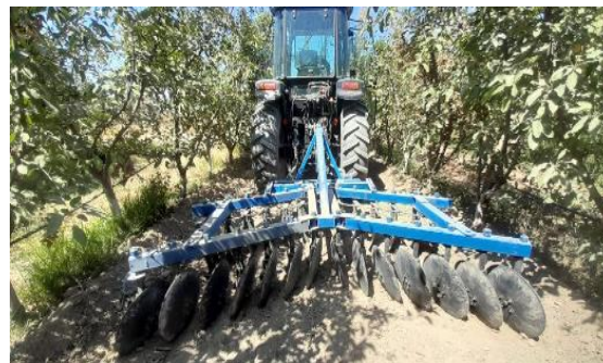
Figure 2. Working process of the device for inter-row cultivation in intensive orchards.
