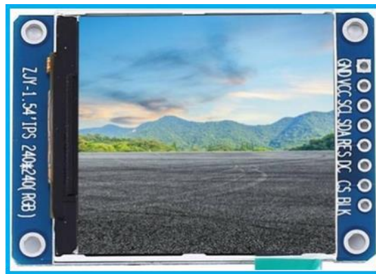
Figure (2.7) 1.3-inch 240x240 RGB TFT IPS LCD display
