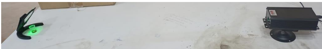
Figure 2: The experimental setup used in the study for irradiating the samples with green semiconductor laser.
