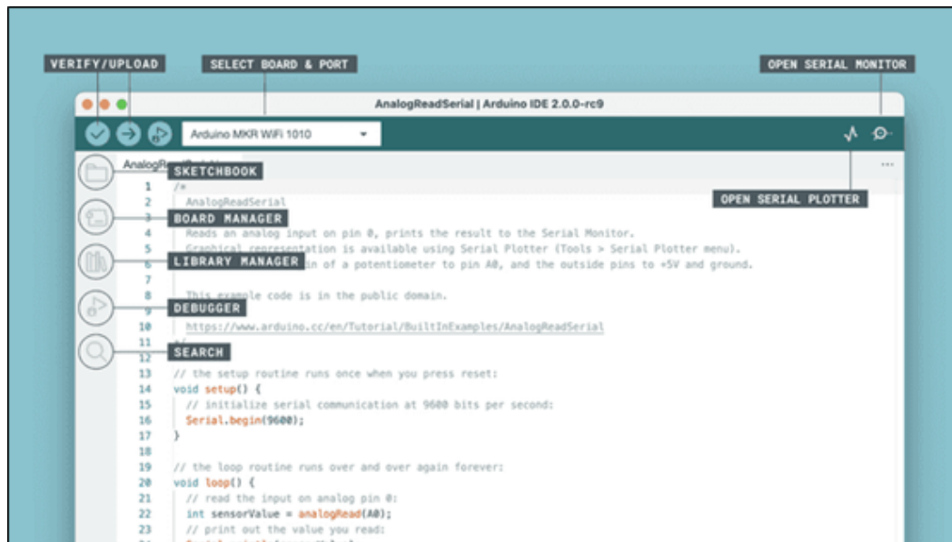
Figure 3-2: Main component of Arduino IDE
