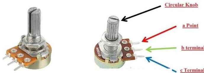
Fig. 10 Structure of variable resistors
