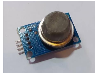
Fig3.10 Air pollutant sensor
