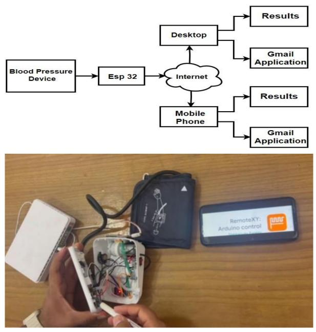
To create a pressure measurement and monitoring system that sends Gmail alerts to a mobile phone, the following steps could be taken:
