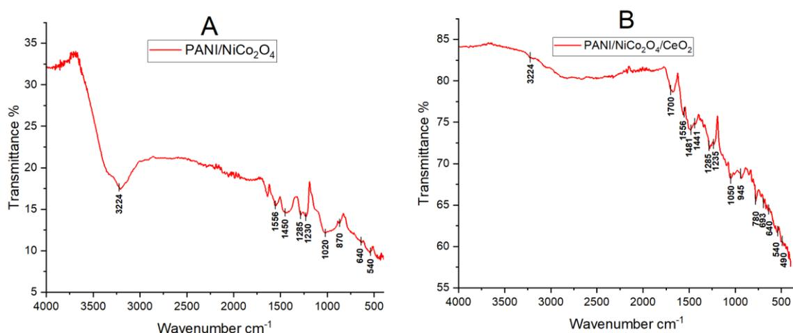
**Figure 2.** A- The FTIR spectra of PANI /NiCo<sub>2</sub>O<sub>4</sub> and B -PANI/NiCo<sub>2</sub>O<sub>4</sub>/CeO<sub>2</sub> nanocomposite
