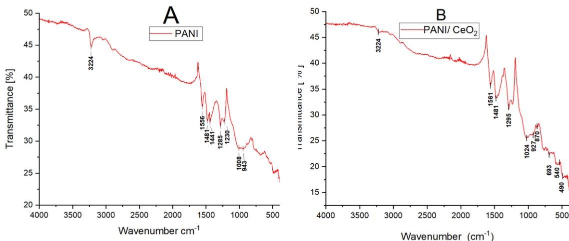
**Figure 1.** A- The FTIR spectra of PANI and B- the FTIR spectra of PANI/ CeO<sub>2</sub>nanocomposite
