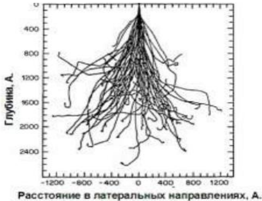
Fig. 3. Trajectory of boron ions in silicon
