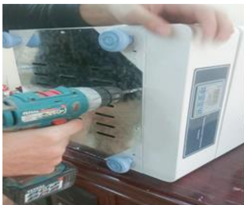
3.1. The picture shows the opening of the base of the incubator
