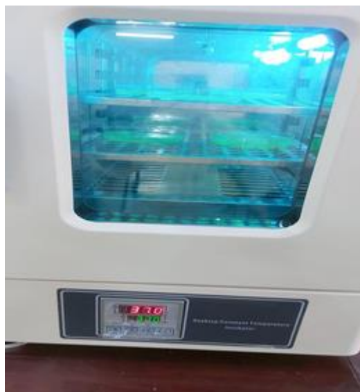
4-1 A picture showing the incubator operating at a temperature of 37 degrees, with samples inside
