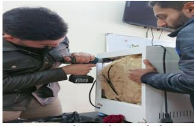
3.5. A picture shows a hole was made in the back of the incubator in order to insert a UV candle
