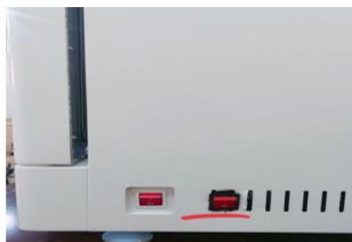
3.4. The picture shows shape of the uv lite power button
