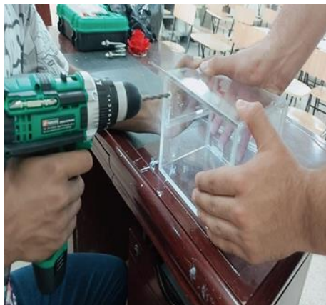
Figure 3-8. The picture shows making holes in the small incubator /chamber
