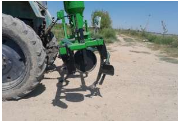
Fig. 2: Machine for deep loosening, cutting roots, and applying fertilizer in pomegranate row spaces.
