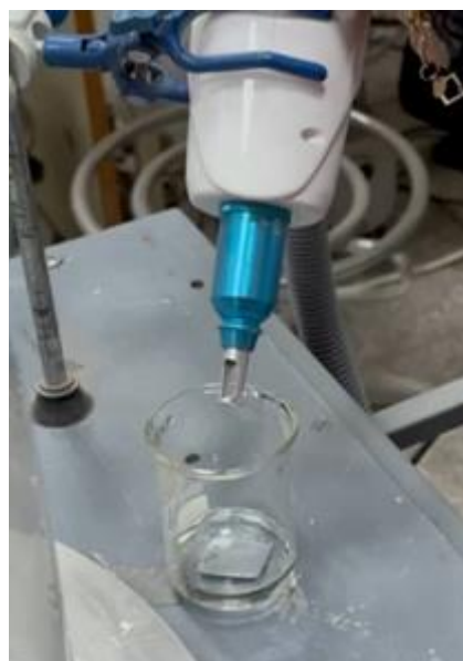
Figure (2.5): Laser targeting of the sample with different powers and pulses, nanoparticles are then formed.
