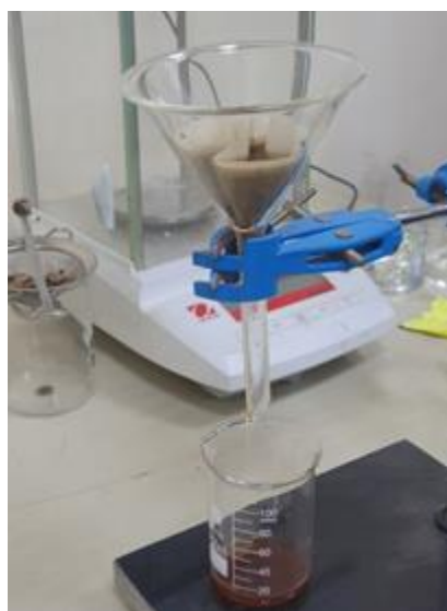
Figure (2.8): Filter the solution using filter papers.
