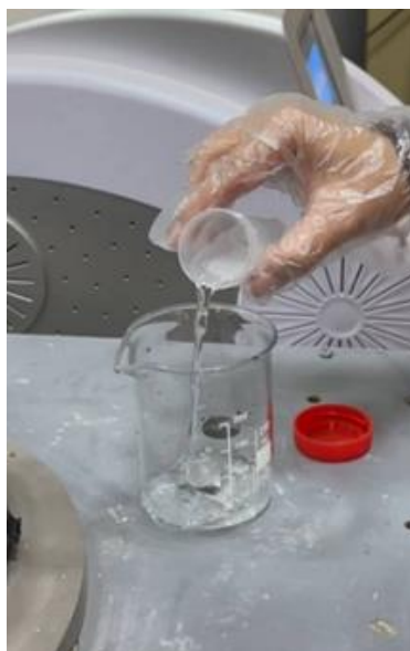
Figure (2.4): The addition of sodium hydroxide solution to the zinc target To make it ready for laser ablation prosess.
