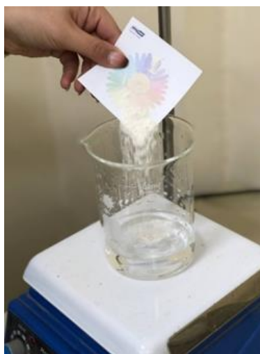
Figure (2.10): Addition of Sodium Alginate into distilled water.
