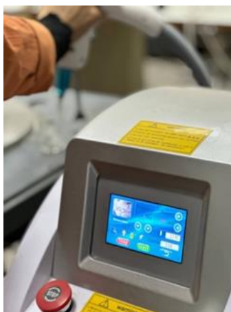
Figure (2.1): AN DYG LASER that was used has a wavelength of 1064nm and a frequency of 8Hz.
