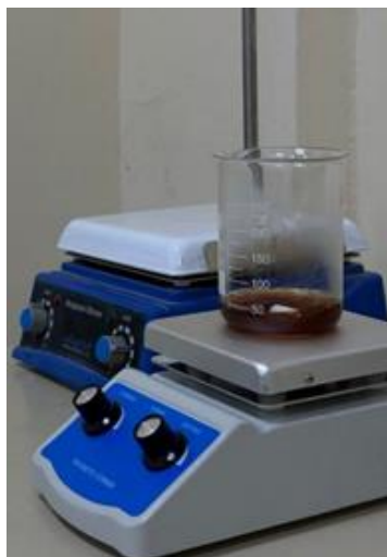
Figure (2.7): The picture shows heating the aloe vera solution at a temperature of 90 degrees
