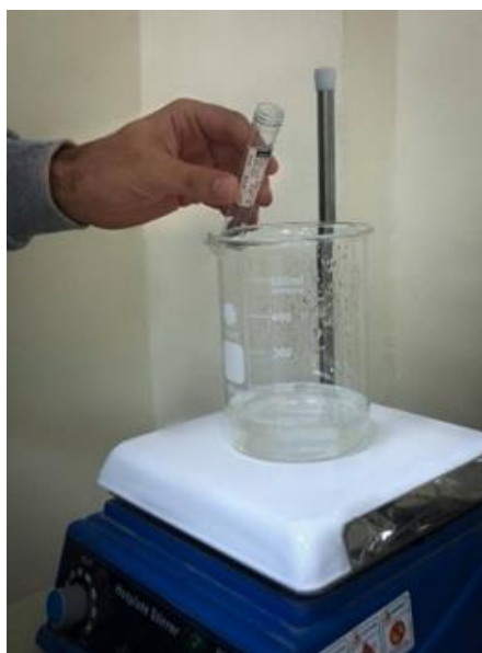
Figure (2.12) The addition of prepared zinc oxide to the sodium alginate solution
