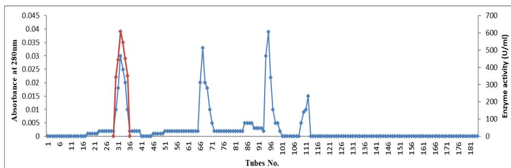
**Figure 9: The chromatogram of Sephadex G-100 for the purification of recombinant lipase**
