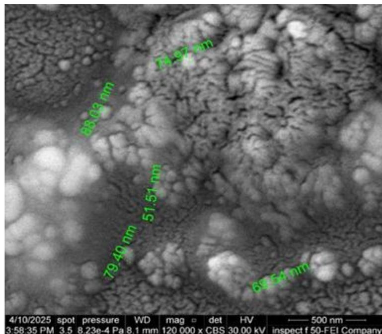
**Figure (3.8)** FESEM analysis of the green synthesized silver nanoparticles.
